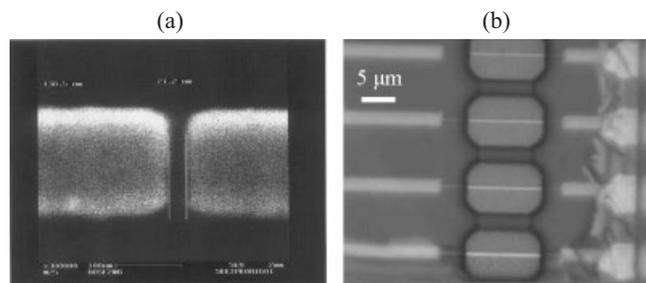
Fig. 1. a) Source and drain electrodes with  $L=27$  nm and  $W=130$  nm. b)  $6\ \mu\text{m} \times 10\ \mu\text{m}$  windows in the photoresist used for the isolation of the transistors (four transistors shown).
