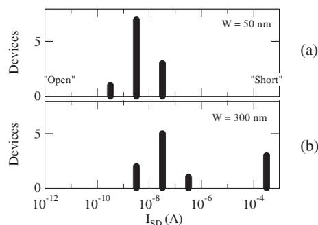
Fig. 3. Histograms displaying the number of devices that exhibit an  $I_{\text{SD}}$  in a certain current range, vs.  $I_{\text{SD}}$ , for  $V_{\text{SD}} = -2$  V,  $V_{\text{SG}} = -4$  V. a)  $L = 30$  nm, and  $W = 50$  nm; b)  $L = 30$  nm, and  $W = 300$  nm. Electrically open devices had an  $I_{\text{SD}} < 10$  pA (no such device shown in this figure) while in shorted devices, the current was limited by the source measure unit to 0.5 mA.
