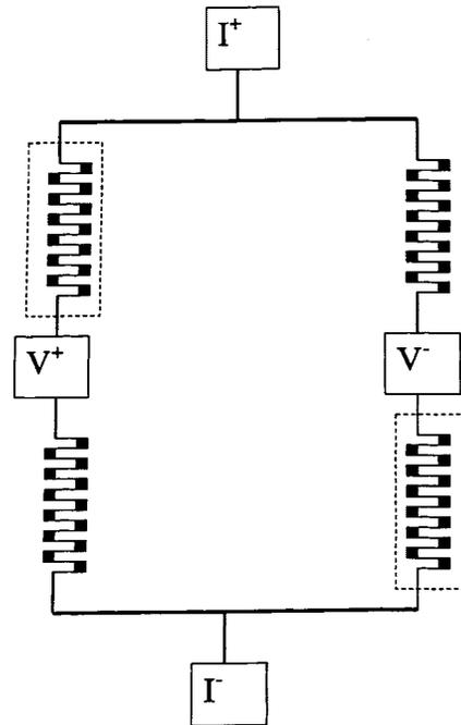
Fig. 1. A simplified schematic of the GMR sensor. There are four GMR resistors, two of which are in-between the flux concentrators (enclosed by the dotted lines). An increase in the dc magnetic field drives the bridge out of balance.
