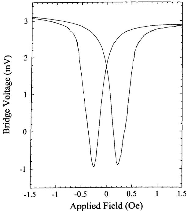
Fig. 2. The bridge voltage,  $V(H)$ , as a function of dc field for the bridge sensor.  $|dV/dH| \approx 16$  mV/Oe near  $H_{dc} = -0.1$  Oe.
