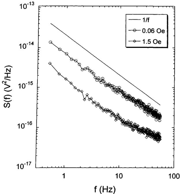
Fig. 5. Power spectra of the fluctuations in the bridge voltage collected at dc fields of 0.06 Oe and 1.5 Oe. The solid line indicates  $S(f) \propto 1/f$ . The Johnson noise for this device is approximately  $4.0 \times 10^{-17} \text{ V}^2/\text{Hz}$ .
