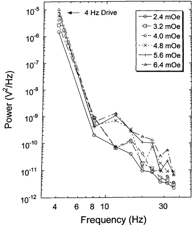
Fig. 6. Noise power at harmonics of the 4 Hz ac magnetic field frequency for several ac field magnitudes.
