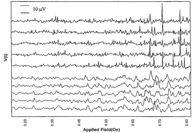
FIG. 3. A comparison of Barkhausen repeatability at driving frequencies of 10 Hz (five upper sweeps) and 100 Hz (five lower sweeps). The data are from the open strip sample, driven with a fixed-amplitude triangle wave.
