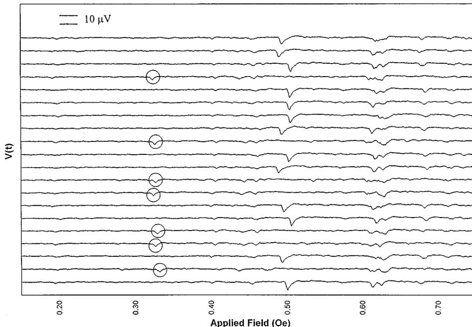
FIG. 4. An example of multiple magnetization paths. The sweeps were taken consecutively fixed sweep parameters. The  $\sim 4 \mu\text{V}$  event circled on the left is directly related to the occurrence of the event, roughly  $8 \mu\text{V}$  in magnitude, that occurs at 0.5 Oe. Also note the relation between the circled event and the event that occurs at around 0.68 Oe.
