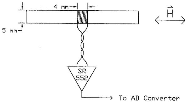
FIG. 2. The experimental setup for the open magnetic sample.
