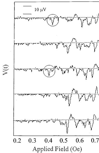
FIG. 5. Another example of two magnetizations paths, from the closed-loop sample. The event circled on the left determines the magnetization path at higher fields.
