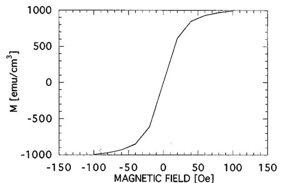
FIG. 1. The entire hysteresis loop, measured using a SQUID magnetometer. The loop width is approximately 0.3 Oe.
